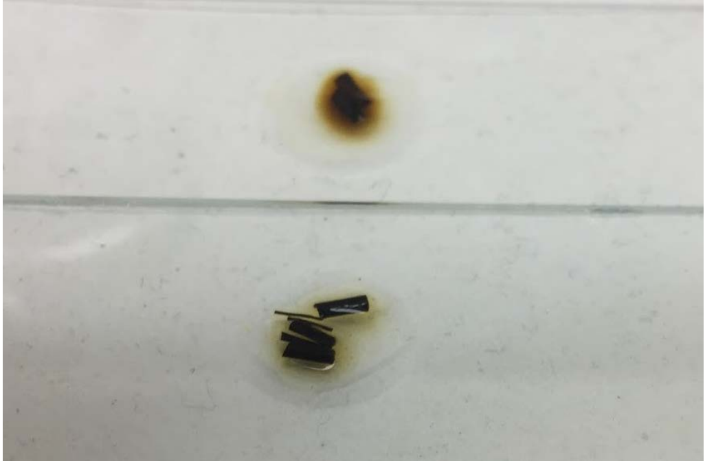
Figure 9: Rhodanine test for hydrolysable tannins: negative. A positive result would have resulted in the formation of a bright pink solution. Basket sample (top), reference sample (bottom).
