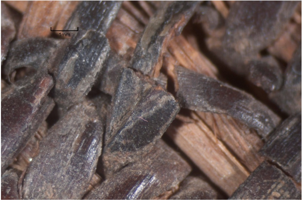
Figure 7: In this photomicrograph it is evident that the dyed Juncus has cracked in several areas.
