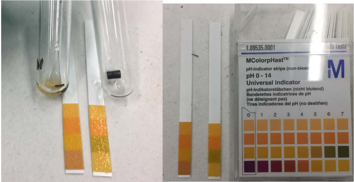
Figure 10 & 11: pH test strips of the basket sample (left) indicated a pH between 3 and 4 while the pH test strip for the reference sample was closer to neutral between 6 and 7.
